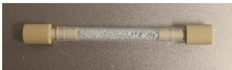
Figure 2: Cadmium reactor before activation
